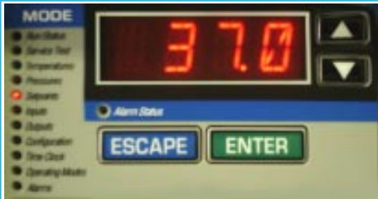
Scrolling marquee diagnostic display and control module.
